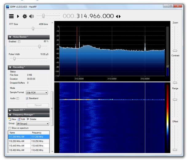
Record the transmission – use the IQ (Baseband) format where possible, as the next step will involve visualizing the transmission in Audacity (free audio software).
