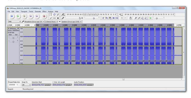
Here, we can visually identify the types of marks (the active area - blue) and spaces (the empty area - grey).
