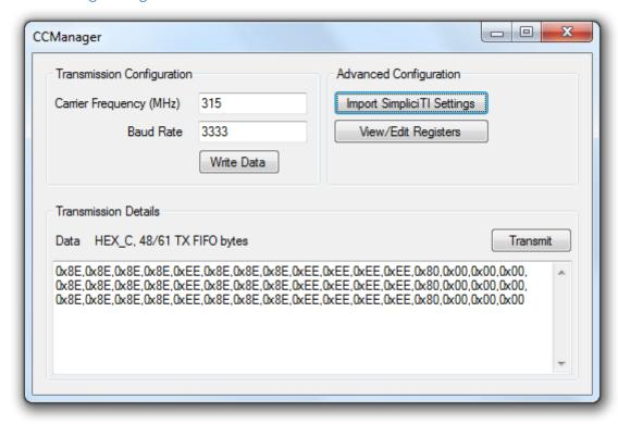
Insert the values for Carrier Frequency, Baud Rate, and Data.
